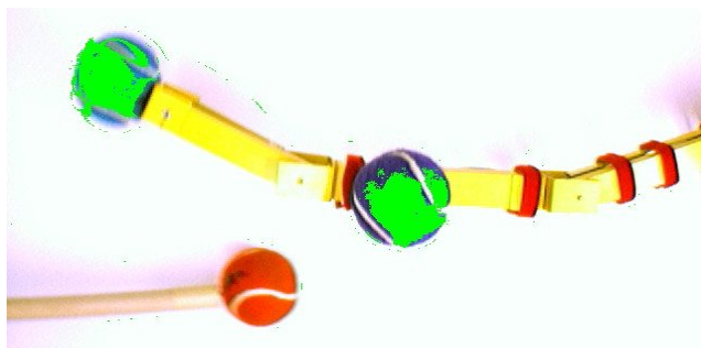
Figure 2: The green pixels indicate which color markers the robot considers “self.” Narcissus recognizes the red anticipatory distractor as “other.”
