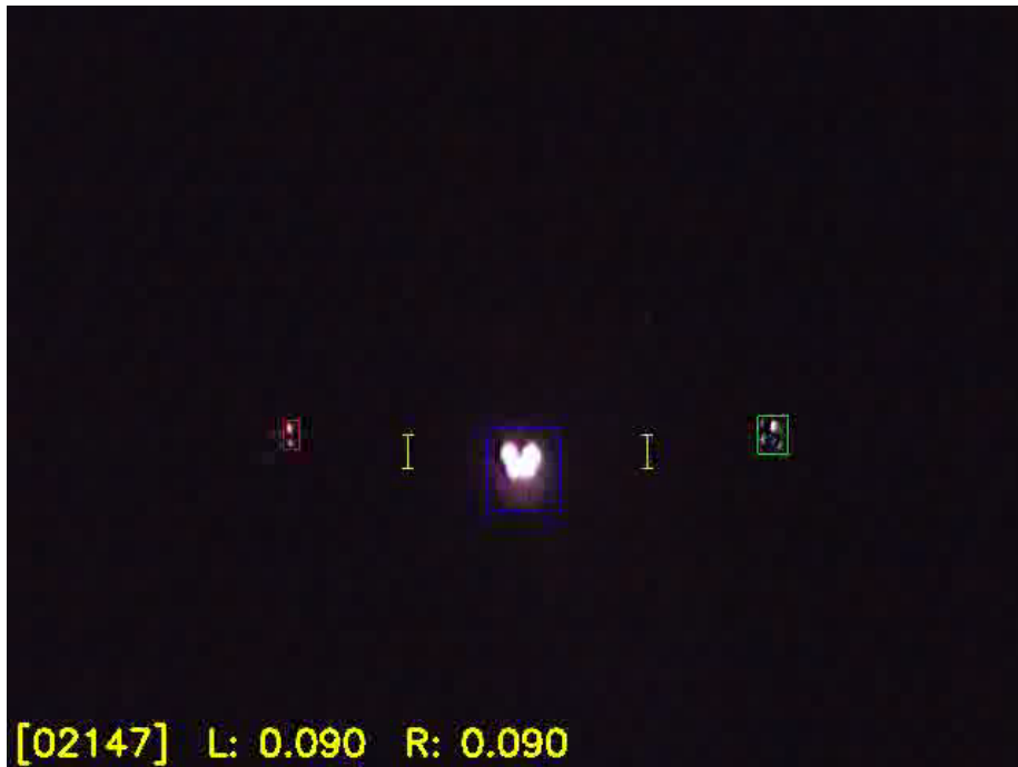
Figure 6: The processed image highlights the left blob in red, the center blob in yellow, and the right blob in green. The yellow lines show the vertical distance between the blobs. The digits along the bottom of the image show the frame counter and the left and right vertical distances.
