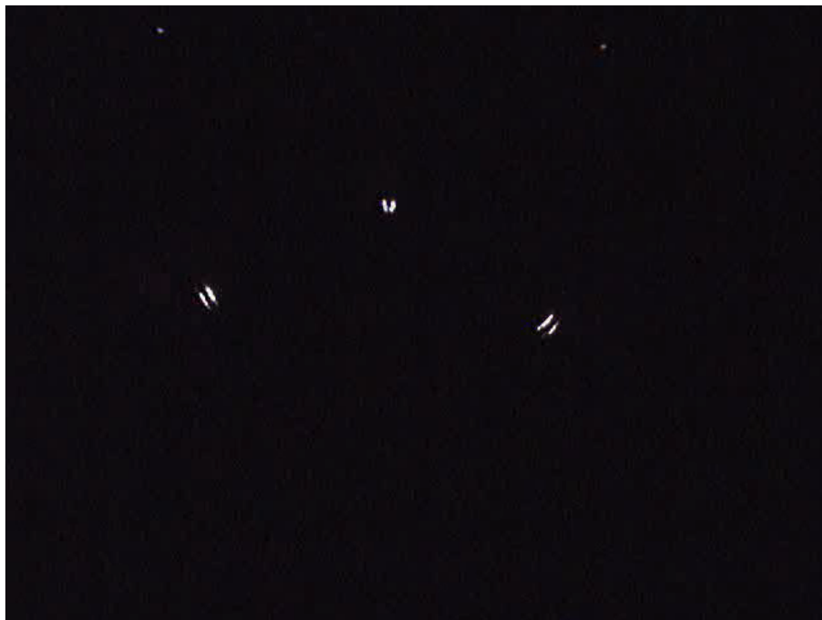
Figure 5: This IR-filtered frame from camera shows Ethan flapping his arms while in the C4 CAVE. The two small white spots at the top of the image are the IR LEDs from the CAVE's tracking system. The three larger blobs are the IR LEDs strapped to Ethan's wrists and back.
